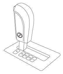
**WARNING:** Always set the parking brake fully and make sure the gearshift is latched in P (Park). Turn the ignition to the off position and remove the key whenever you leave your vehicle.
